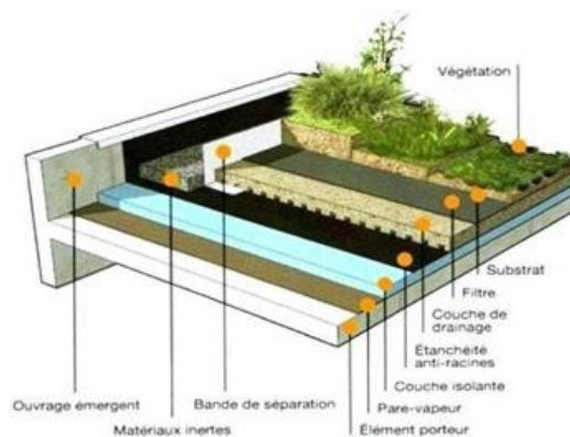
Figure 14. Structure of a green roof, www.liaisonveg.etal.com .
