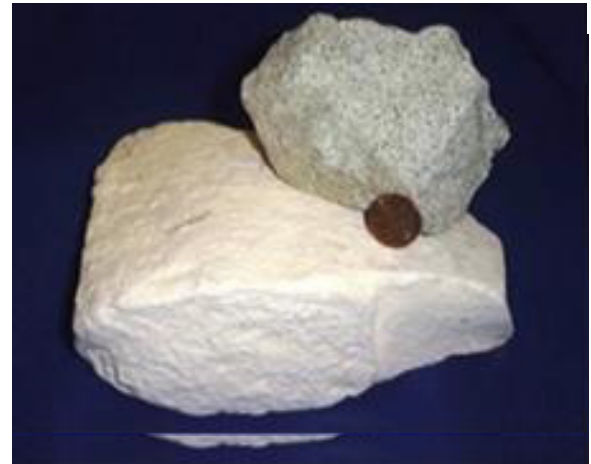
Photo 12. A zeolite is a rock formed from a microporous aluminosilicate skeleton, the voids of which optimise the adsorption and biodegradation processes of the reed root system. Source www.amethyst.it .
