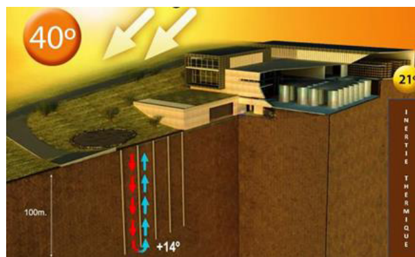
Figure 20. Application of geothermal energy in the cellars to take advantage of the thermal inertia of the subsoil (coolness in summer and warmth in winter), Bodegas Regalia de Ollauri in La Rioja, Spain, www.marquesdeteran.com .
